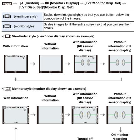
\* It is displayed when [Monitor Info. Disp.] in the [Custom] ([Monitor / Display]) is set to [ON]. You can touch the desired item and change its setting directly.
