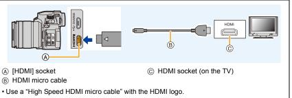
Cables that do not comply with the HDMI standards will not work.
