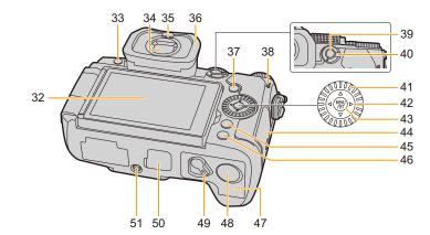
32 Touch screen (P52)/monitor (P318) 33 [LVF] button (P42)/[Fn3] button (P60) 34 Viewfinder (P42, 338) 35 Eye sensor (P42) 36 Eye cup [ ] (Playback) button (P184) 37 38 Speaker (P230) 39 [AF/AE LOCK] button (P110) 40 Focus mode lever (P93, 95, 107) 41 Control dial (P47) Cursor buttons (P48)/ ▲ Fn button (Fn9) (P60) 42 Fn button (Fn10) (P60) ▼ Fn button (Fn11) (P60) [ ] (AF Mode) button (P93)
