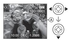
The motion picture recording time (A) is displayed on the screen. After playback starts, the motion picture recording time disappears and the elapsed playback time is displayed on the bottom right of the screen.
