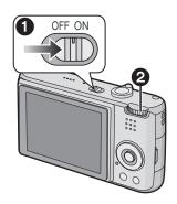
2 Aim the AF area ① to the point you want to focus on and then press the shutter button halfway.
