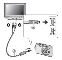
1 Connect the AV cable (a) (supplied) to the [AV OUT] socket on the camera.
