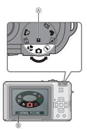
• The above screen (B) appears on the LCD monitor if the mode dial is rotated. (P21) The mode currently selected appears on the LCD monitor when the camera is turned on
