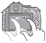
This is used to move the AF area, operate the slide bar etc.
