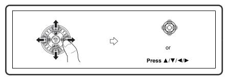
Even when the camera is operated using the touch panel, it is possible to operate with the cursor button and [MENU/SET] button if a guide like the one shown on the right is displayed.
