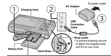
SD Memory Card (optional) The following cards, which conform to the SD standard, can be used with this unit.
