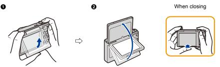
Flip up the bottom of the monitor lightly to open.Adjust the angle of the monitor.
