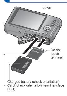
Set the camera ON/OFF switch to OFF Slide to the [OPEN] position and open the lid
