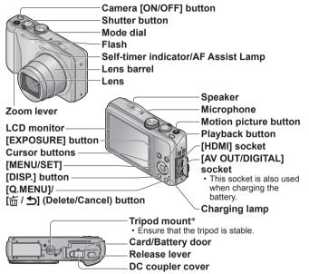
Do not attach to a tripod with a 5.5 mm (0.22 inch) or longer screw. Doing so may damage this unit.
