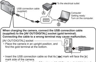
Always check the direction of the pins and hold the plug straight to insert or remove it. (If the cable is inserted in the wrong direction, the pins could become deformed and cause faulty operation.) Also, do not insert into the wrong socket. Doing so may cause damage to this unit.
