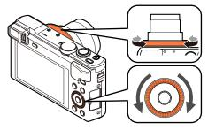
(In [Program AE] mode, the control ring is assigned to [Step Zoom].)
