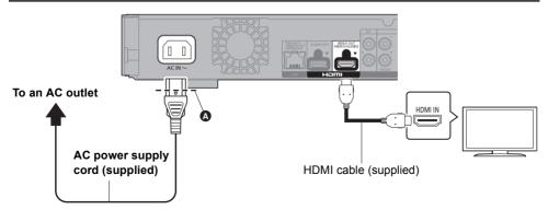
• Insert the AC power supply cord up to (a), a point just before the round hole.
