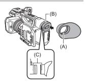
Attach the eye cup so that the ridge inside it is aligned with the groove on the eye cup mount.
