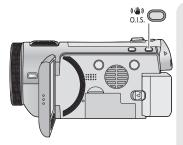
Optical image stabilizer button Pressing the button changes the Optical image stabilizer setting. (Motion Picture Recording Mode)  $((()) \rightarrow ((())) \rightarrow (())) \rightarrow OFF$
