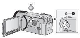
To turn off the power Hold down the power button until the status indicator goes off.
