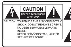
The lightning flash with arrowhead symbol, within an equilateral triangle, is intended to alert the user to the presence of uninsulated "dangerous voltage" within the product's enclosure that may be of sufficient magnitude to constitute a risk of electric shock to persons.
