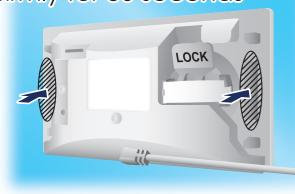
14. Attach the cover (1) Tuck removal tab inside 2 Attach the cover
