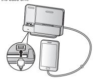
■ If your smartphone's USB port is located at the center of its bottom panel You can also run a USB cable (not supplied) through the cable slot (♠) and place your smartphone on the base unit for charging.
