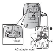
Insert the hooks on the wall mounting adaptor into holes (a) and (b) on the base unit
