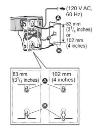
To remove the wall mounting adaptor While pushing down the release levers (①), remove the adaptor (②).
