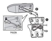
Insert the hooks on the wall mounting adaptor into the holes (a) and (3) on the base unit.
