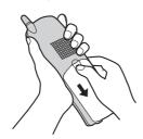
2 Insert the battery (1), and press it down until it snaps into position (2). Then close the handset cover.
