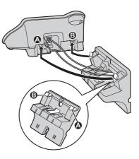
**4** Adjust the adaptor to hold the base unit, then push it in the direction of the arrow until it clicks into place.
