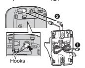
Insert the hooks on the wall mounting adaptor into holes (4) and (3) on the base unit.
