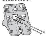
Tuck the telephone line cord inside the wall mounting adaptor (●). Connect the AC adaptor cord and telephone line cord (②).
