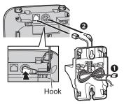
Insert the hooks on the wall mounting adaptor into holes (2) and(3) on the base unit.
