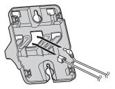
2 Tuck the telephone line cord inside the wall mounting adaptor (●). Connect the AC adaptor cord and telephone line cord (●).
