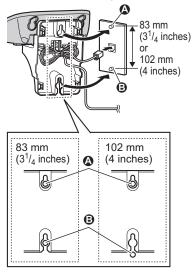
To remove the wall mounting adaptor While pushing down the release levers (①), remove the adaptor (②).
