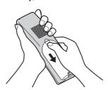
2 Insert the battery (1), and press it down until it snaps into position (2). Then close the handset cover (3, 4).
