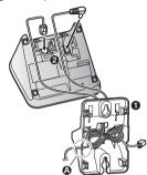
Insert the hooks on the wall mounting adaptor into holes (A) and (B) on the base unit.
