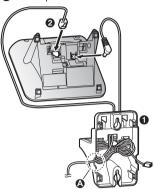
3 Insert the hooks on the wall mounting adaptor into holes (**(A)**) and (**(B)**) on the base unit.
