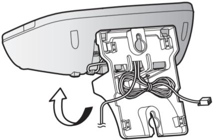
**5** Mount the unit on a wall then slide down to secure in place.
