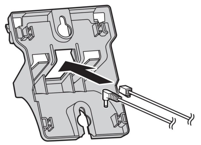
2 Tuck the telephone line cord inside the wall mounting adaptor (1). Connect the AC adaptor cord and telephone line cord (2).
