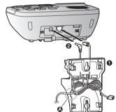
3 Insert the hooks on the wall mounting adaptor into holes ((A)) and ((B)) on the base unit.
