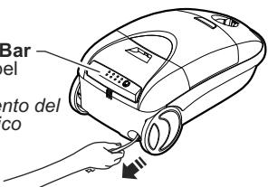
➤ Pull cord out of canister to desired length.
