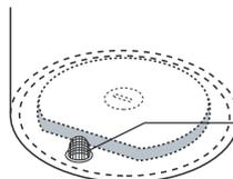
The filter can be removed by pulling firmly on it.
