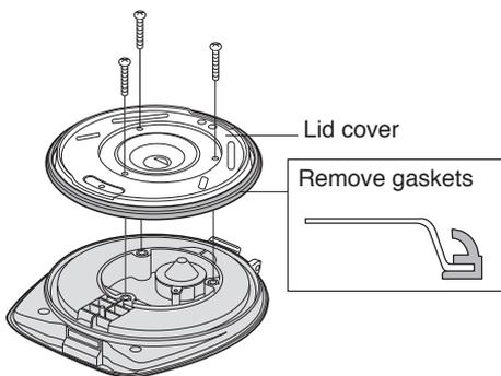
Remove lid, unscrew 3 tapping screws and remove the lid cover.
