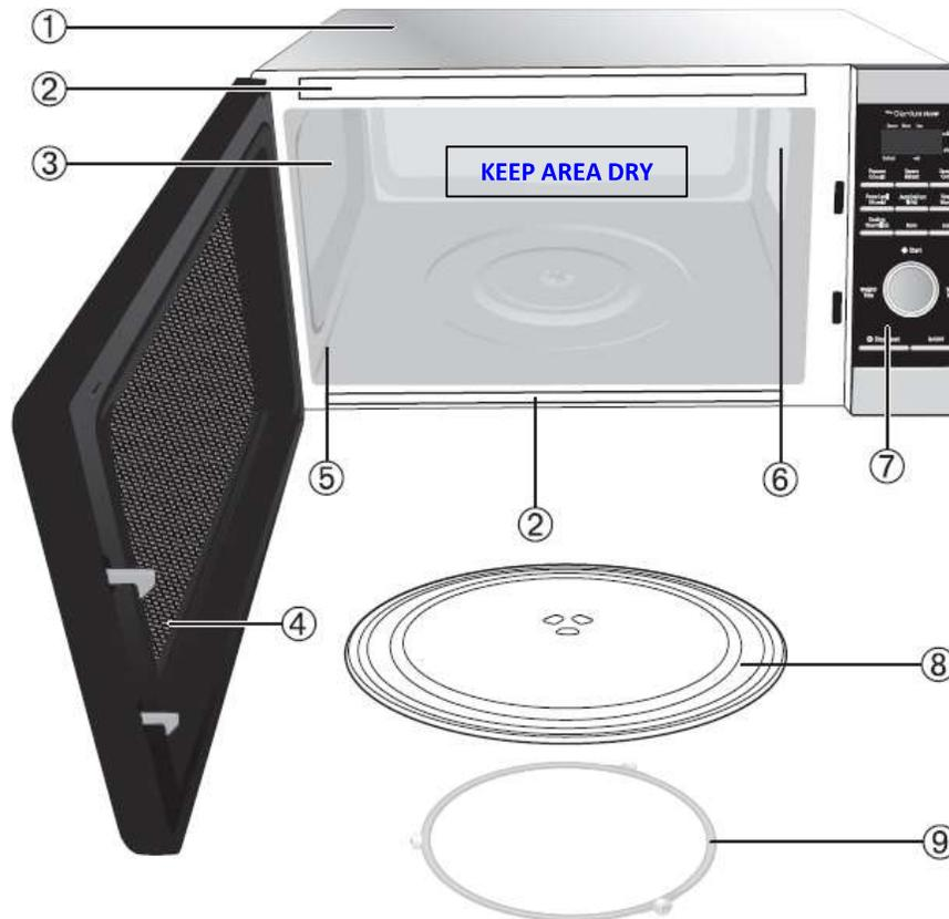
**6. Wave Guide Cover:** Do not remove Wave Guide Cover. It is important to keep cover clean in the same manner as the inside of the oven.
