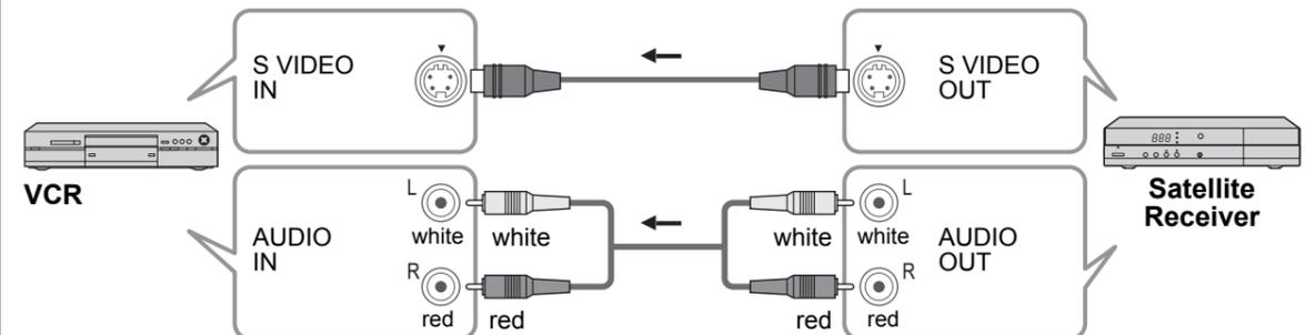
● The S Video input will override the composite video signal when S Video cable is connected. Connect either S Video or Video cable.
