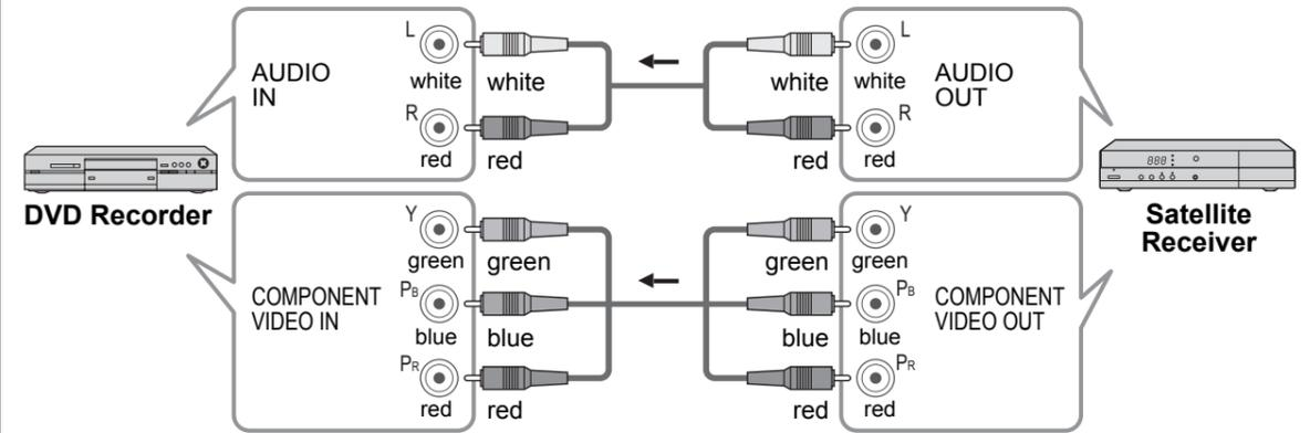
● Satellite Receiver may also be connected to COMPOSITE or S VIDEO terminals. (see below)
