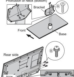
Hole for pedestal installation Bracket Base Work on a flat surface
