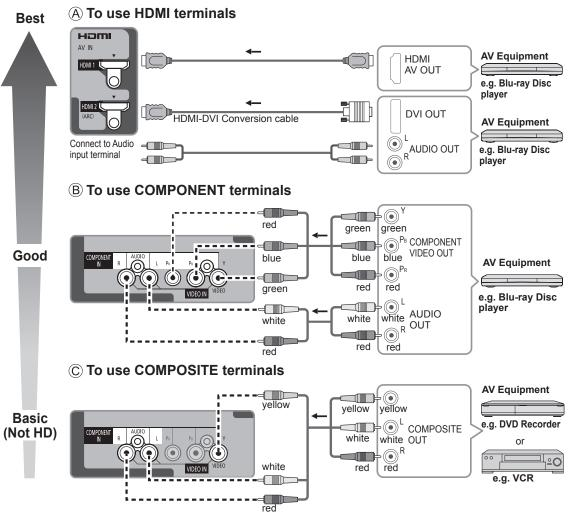
The Green terminal is shared for both the COMPONENT and COMPOSITE (VIDEO IN) connection.
