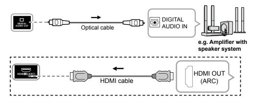
HDMI connection is available if connected audio equipment has ARC (Audio Return Channel) function.
