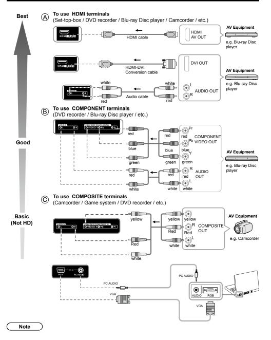
The Green terminal is shared for both the COMPONENT and COMPOSITE (VIDEO IN) connection. When
