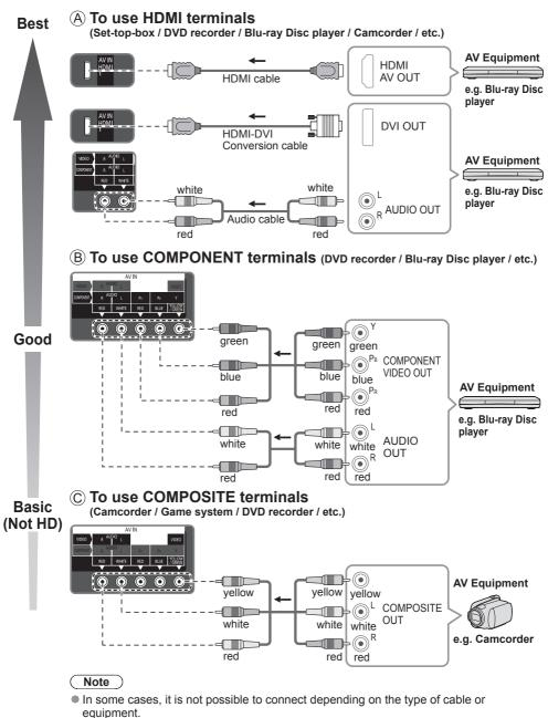
The Green terminal is shared for both the COMPONENT and COMPOSITE (VIDEO IN) connection. When using COMPOSITE (VIDEO IN) connection, the Yellow connector (Video) should be inserted into Green connection.
