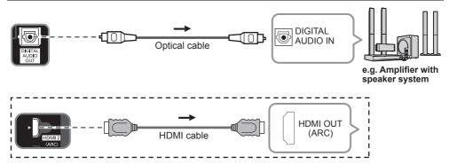
HDMI connection is available if connected audio equipment has ARC (Audio Return Channel) function.
