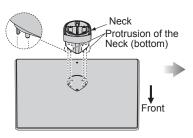
(2) Turn the stand over and fix stand neck securely with assembly screws.
