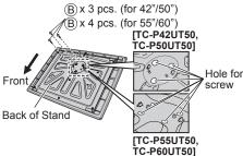
Make sure that the bracket is anchored before fixing the screws.
