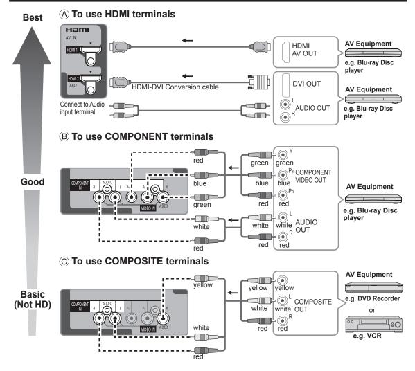
• The Green terminal is shared for both the COMPONENT and COMPOSITE (VIDEO IN) connection. When using COMPOSITE (VIDEO IN) connection, the Yellow connector (Video) should be inserted into Green connection.
