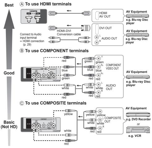
The Green terminal is shared for both the COMPONENT and COMPOSITE (VIDEO IN) connection. When using COMPOSITE (VIDEO IN) connection, the Yellow connector (Video) should be inserted into Green connection. (Watching content from external devices (p. 19))
