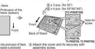
③ Attach the Bracket to the protrusion of Neck. Make sure that the bracket is anchored before fixing the screws. Fix securely with assembly screws (4 screws)
