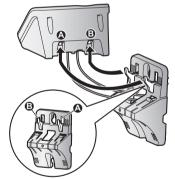
4 Adjust the adaptor to hold the base unit, then push it in the direction of the arrow until it clicks into place.
