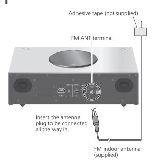
• Tape the antenna to a wall or column at the position with the least amount of interference.
