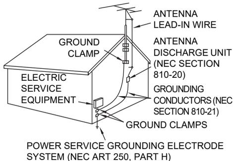
19) An outside antenna system should not be located in the vicinity of overhead power lines, other electric light, power circuits, or where it can fall into such power lines or circuits. When installing an outside antenna system, extreme care should be taken to keep from touching such power lines or circuits as contact with them might be fatal.
